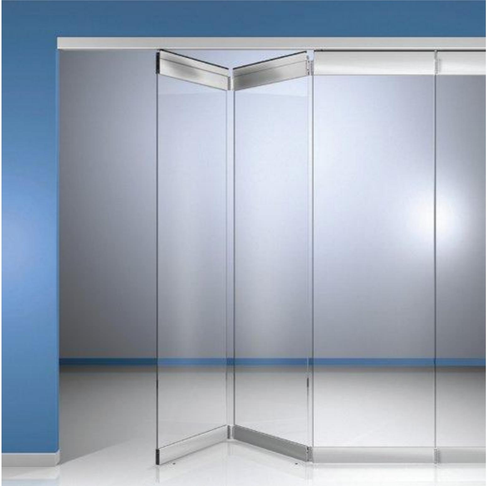
The size of each door varies and can reach up to 80cm wide and up to 300cm height. On top and Bottom glass doors are equipped with aluminum Profile . According to the glass holding patent system Sealing between the doors is achieved with Transparent polycarbonate or aluminum profiles That bear synthetic insulating brush. All top and Bottom aluminum profiles are equipped with the same brush in order to satisfactory seal the minor gaps.
